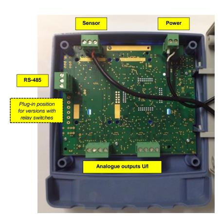
**Remark:** If more than 1 probe is connected, the single wires can be fixed in parallel in the same screw terminal.
