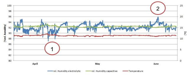
Peaks (1) and (2) originated from problems with the humidification/dehumidification installation, which was not detected by the building technology.
